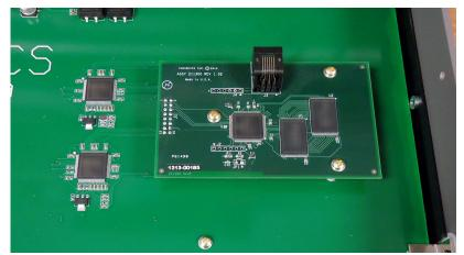
Mounting standoffs are already in place on the DAVID IV main board. Simply plug the accessory board squarely onto the mainboard header strip so that the three mounting holes line up.
